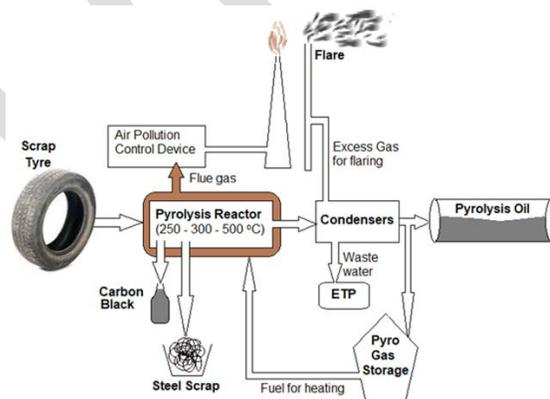
**Fig. 1:** Schematic diagram of waste tyre pyrolysis process
